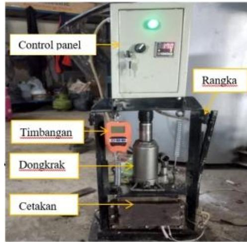
Gambar 4. Mesin *hot press*
