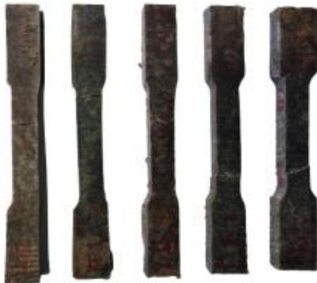
Gambar 8. Sampel uji tarik (mengikuti standar ASTM D639)
