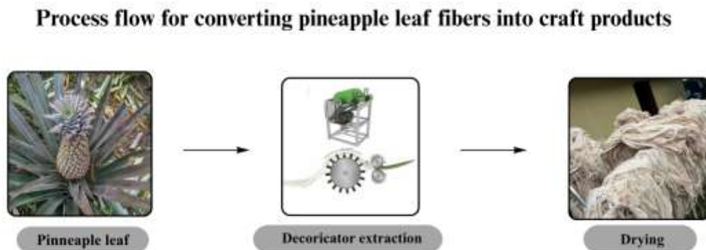
Figure 2. Implementation of Stages of Processing Flow of Pineapple Leaf Waste into Cellulose Fiber
