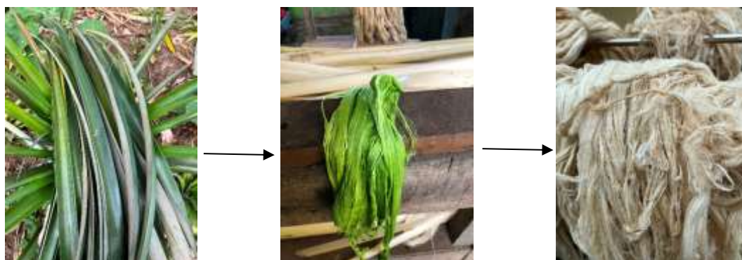
Figure 6. The Stages of Pineapple Leaf Fiber Processing
