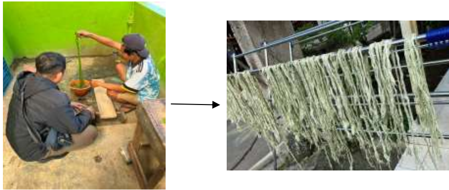
Figure 3. Washing and Drying of Pineapple Leaf Fibers
