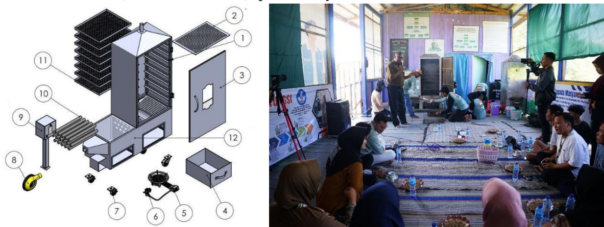
(a) Parts of fish dehydrator machine (b) Demo and training of fish dehydrator machine Caption of (a): (1) Fish processing room, (2) charcoal filter, (3) door, (4) biomass container, (5) gas stove, (6) solenoid valve, (7) caster wheel, (8) blower, (9) control panel, (10) hot air pipe, (11) fish container, (12) combustion chamber
