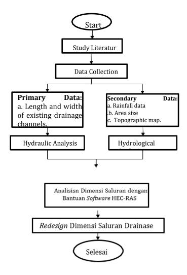
The required data consisted of primary and secondary data. The primary data included existing drainage data such as channel width and channel depth, while the secondary data included hydrological analysis data such as rainfall data from rain gauge stations and the total area of Margahayu Housing Complex in Bekasi City, which is approximately 330,000 m<sup>2</sup>.
