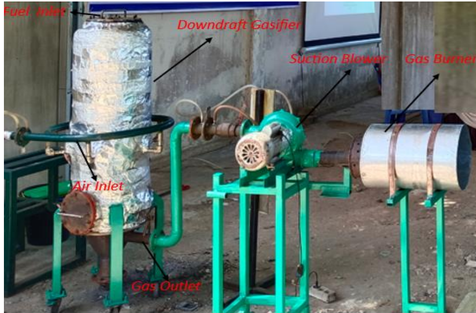
Figure 5. Downdraft Gasifier Gasification System Down to Community Service Location
