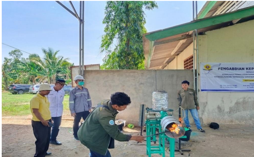
Figure 11. The ignition process of the formed gas fuel
