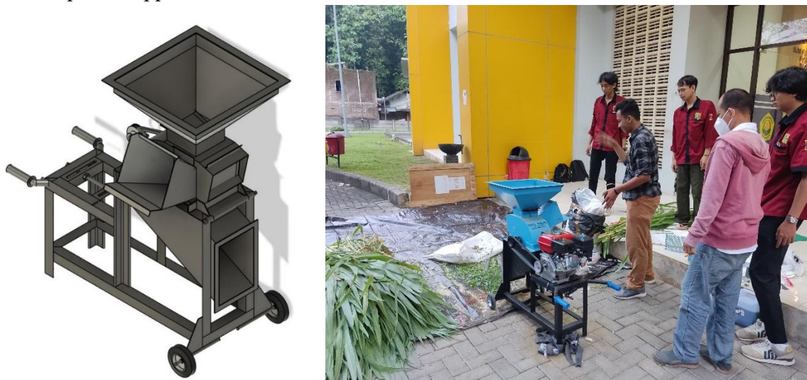
Figure 1. The chopper machine: (a) design, (b) performance testing
