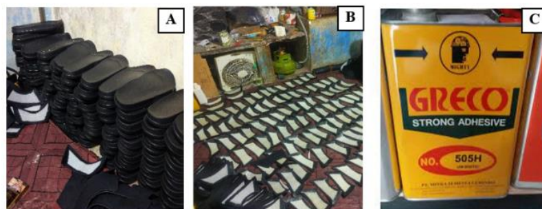
Figure 1. Materials for slippers (A) Mitsol, (B) Upper, (C) Lem
