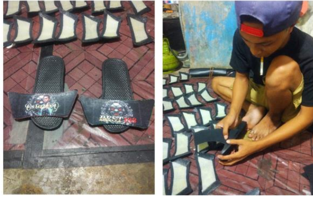
Figure 2. Upper Installation Process on Mitsol
